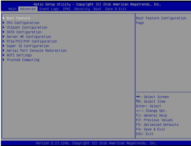
**Warning:** Take caution when changing the Advanced settings. An incorrect value, a very high DRAM frequency, or an incorrect DRAM timing setting may make the system unstable. When this occurs, revert to the default to the manufacture default settings.
