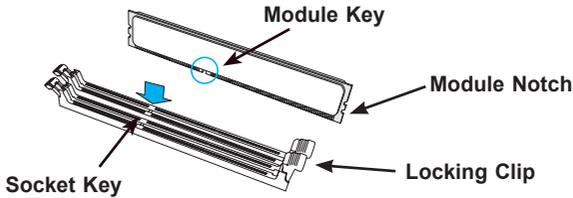
2. Install the DIMM module straight down into the socket until it is securely seated in the socket. The side clips will automatically lock the module into place.
